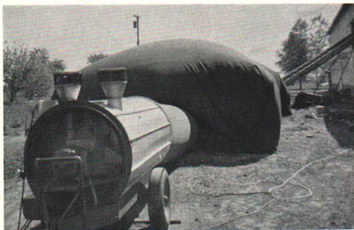
FIG. 15.—Drying platform loaded with baled hay and with fan running.
