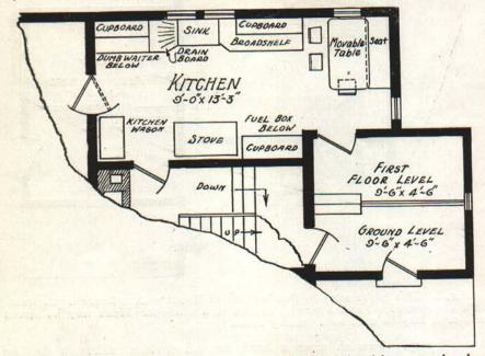
Fig. 4. A variation of the floor plan shown in Fig. 2. A breakfast noow has been added and the enclosed back room shifted so there is no outside cellar door.
