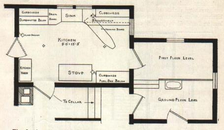
Fig. 2. A compact kitchen having built-in equipment. The work shelf and sink are close together, with the range but a step away. Note that the dumb waiter and dish cupboard are close to the dining room.
