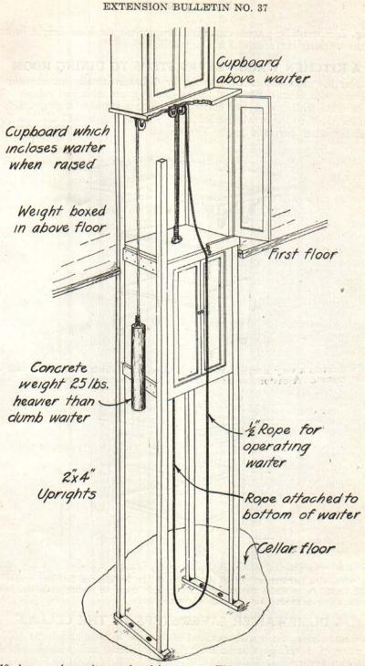
Fig. 10 shows a dumwaiter enclosed in a case. This type is very satisfactory and can be installed by the local carpenter.
