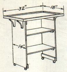
Fig. 8 illustrates a very simple, home made wheel tray which is equipped with common castors. A castor having a 3-inch wheel with rubber tire is preferable.
