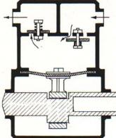
Fig. 12. - Diaphragm pump.
