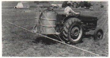
Fig. 4. - Tractor-mounted weed sprayer.
