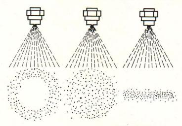
Fig. 14. – Three common boom type nozzle spray patterns – L to R – Hollow cone, solid cone, fan.
