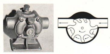
Fig. 9. - Flexible impeller pump.
