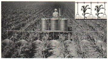
Fig. 16. - Drop pipes for corn herbicide application.
