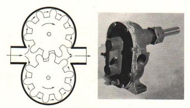
Fig. 8. - Gear pump.
