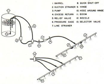
Fig. 6. - Layout of a boom weed sprayer.
