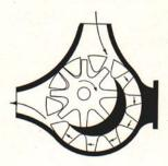
Fig. 13. - Internal idle gear pump.
