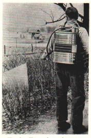
Fig. 1. - Compressed air hand sprayer.
