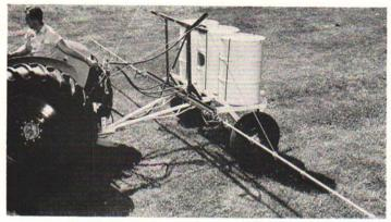
Fig. 5. - Trailing type weed sprayer with PTO pump.
