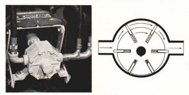
Fig. 11. - Sliding vane impeller pump.
