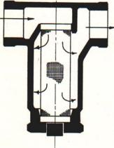
Fig. 23. - One type of line strainer.
