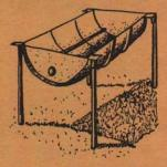
Fig. 2. Pit made from steel drum.
