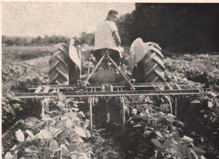
Fig. 16. These soybeans were planted with the one-row planter shown in Fig. 15, and cultivated two rows at a time as shown here.
