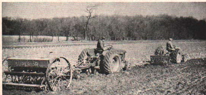
Fig. 11. Don Pace, Calhoun County, Michigan, has figured how to plow and plant oats in one operation. The rear plow has three 14-inch bottoms and a tandem packer, with the eleven-hole (7-inch spacing) grain drill attached to the outer end of the packer frame. Ahead is a two-bottom 16-inch plow with packer. Oats are fertilized and legume is seeded in one operation, leaving no tractor wheel marks.
