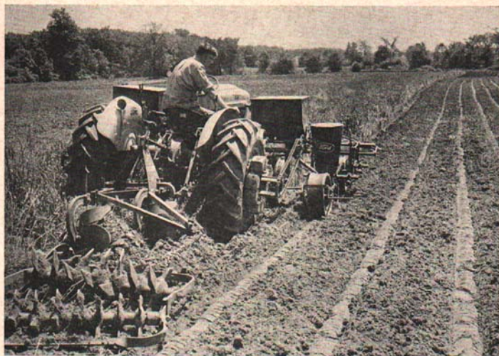
Fig. 15. This equipment applies fertilizer to be plowed under (left hopper), fits the soil with a revolving bladed tiller, applies fertilizer beside the row, and plants soybeans, all in one operation. The 30-inch rows were well enough spaced to allow the use of a two-row cultivator. For planting corn, a three-bottom plow was used and a pre-emergence weed sprayer was added. This machine is still in the experimental stage, but it has operated quite satisfactorily.
