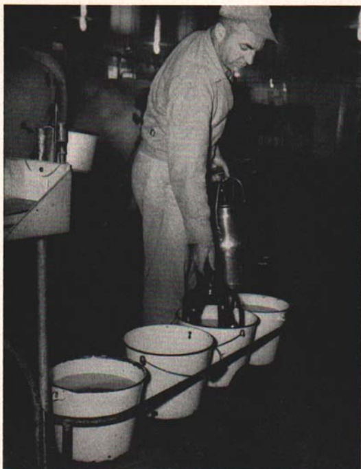
Fig. 5. Rinse the machine with cold or lukewarm water immediately after milking each cow. Then dip in a sanitizing solution.
