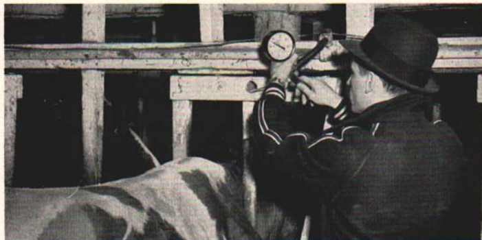
Fig. 6. Checking the vacuum pressure is necessary to maintain proper milking machine operation.
