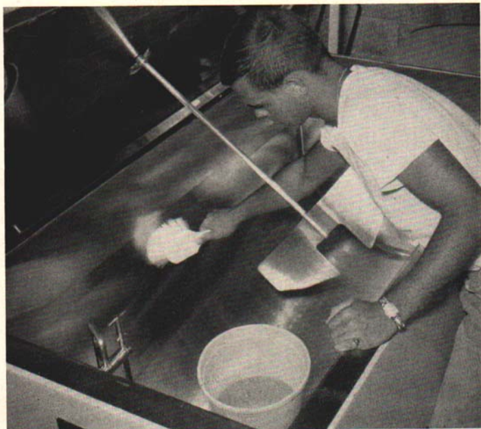
Using a soft brush and a plastic pail while washing the bulk tank prevents scratches on the stainless steel surface inside the tank.
