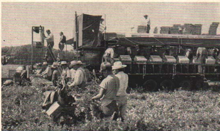
Fig. 14. Florida-built celery harvester in operation in a Kent County field. All operations—cutting, trimming, washing, grading, and packing—are included. It requires nearly 100 man-hours to pack 10,000 stalks.
