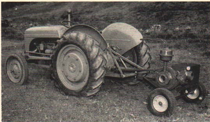
Fig. 2. Trailer mounted PTO driven pump with bevel gear type speed increaser.
