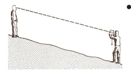
Fig. 3 — Two people or two posts may be used to determine slope with the slope finder.
