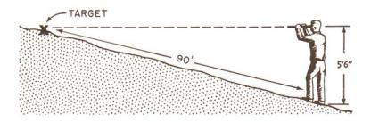
Fig. 4.— In this sketch, percent slope is being estimated with a hand level. The man has established that his eye or line of sight is 5.5 feet above the ground when he stands erect. He sights uphill through the level to an object which he has placed on the ground for a target. He watches the bubble in the level
