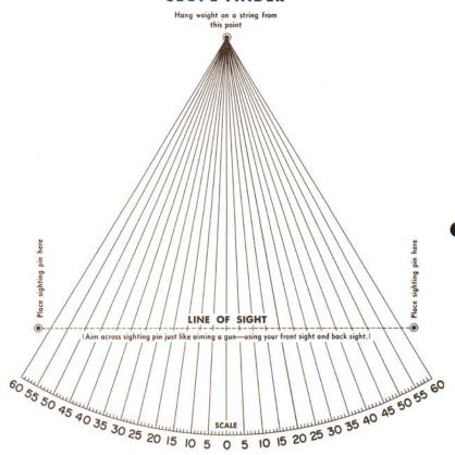
Read percent of alope directly on this scale. At this point where string rests on scale, the number indicates percent of slope, or the number of feet of rise or fall in 100 feet.
