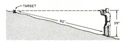
Fig. 4.— In this sketch, percent slope is being estimated with a hand level. The man has established that his eye or line of sight is 5.5 feet above the ground when he stands erect. He sights uphill through the level to an object which he has placed on the ground for a target. He watches the bubble in the level
