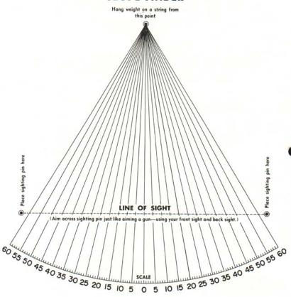
Read percent of slope directly on this scale. At this point where string rests on scale, the number indicates percent of slope, or the number of feet of rise or fall in 100 feet.
