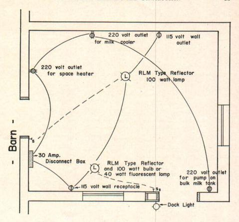
Fig. 8. Suggested wiring diagram for a farm milkhouse.
