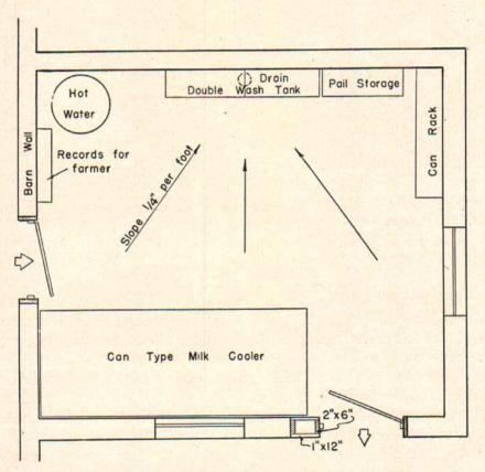
Fig. 4. Suggested layout for milkhouses with doors on adjoining sides, equipped with can-type coolers. (See Table 1 for dimensions.)
