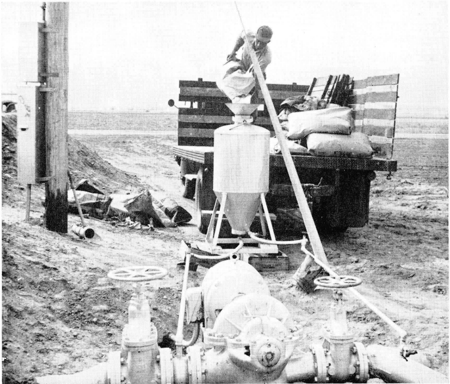
Fig. 6. One type of commercial fertilizer applicator which utilizes a pressure difference for feeding the solution into the sprinkler system.
