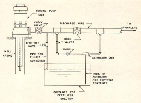
Fig. 8. Arrangement of the equipment necessary when an aspirator unit is used to suck the fertilizer solution into the pipeline.
