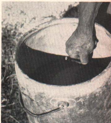
Fig. 5. After establishing the water measure to be used, mark it on the inside of the pail with a heavy pencil. Then use only for water.
