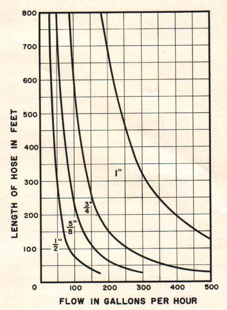
Fig. 5. "Hose selection chart." Use in the same manner as Fig. 4. (Both Figs. 4 and 5 are based on data originally compiled by J. E. Christiansen, Dean of Engineering, Utah State College, and used with his permission.)
