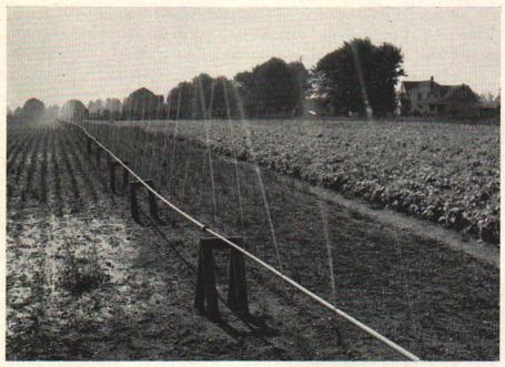
Fig. 6. "Oscillating pipe" supported by sawhorses, in use for truck-garden irrigation. A motor at one end rotates the entire lateral through a quarter-circle for consistent water distribution.
