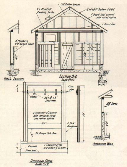
Fig. 8b. End section and construction details for individual bull barn.
