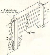
Fig. 4. The pipe and concrete post fence recommended.
