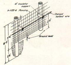
Fig. 7. Woven wire fence, reinforced by an electrified wire.
