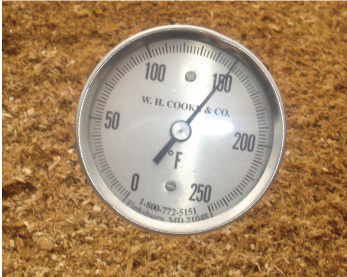
Photo 7. Long-stem thermometer (available commercially as “compost” or “windrow” or “hay” thermometer) is used to monitor internal temperature.
