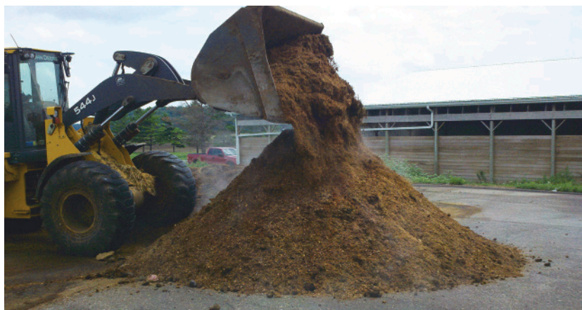
Photo 2. Utilizing a front-end loader for turning, moving and mixing.
