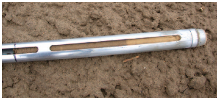
A probe for sampling soil.
