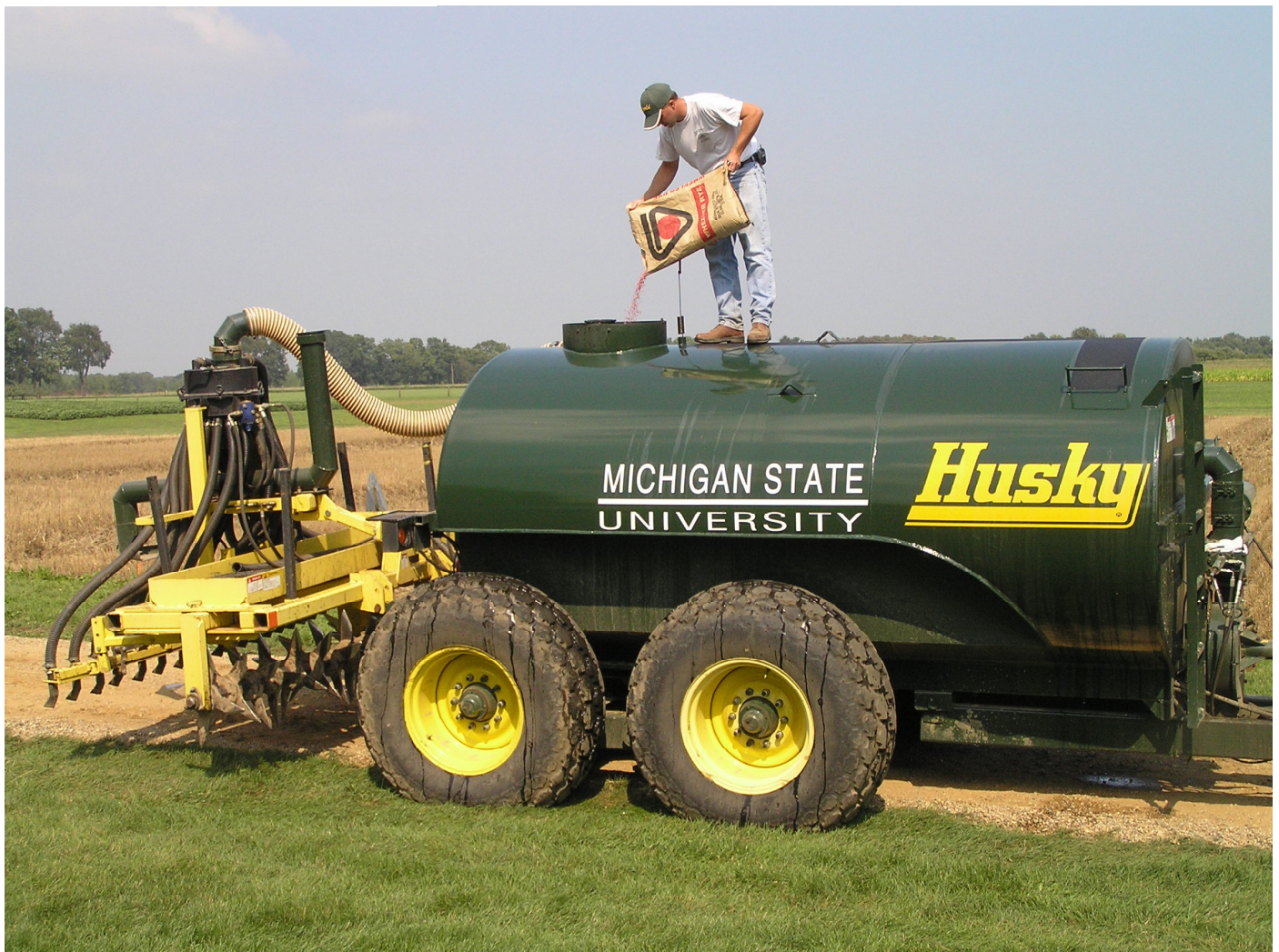
Fig. 1. Seed is mixed directly in the tank and applied with the manure slurry.
