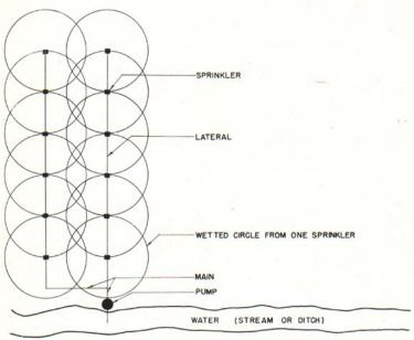
Fig. 4. Field layout for a portable system.
