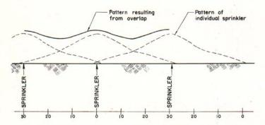
Fig. 7. Distribution of water from overlapping sprinklers.
