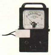
Fig. 2. Bouyoucos soil-moisture meter with plaster-of-paris block.
