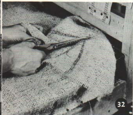
FIGURE 31. Mark and slip-tack (placing in tacks only partially for a temporary tacking) centers of burlap on all sides. Check that the grain of the fabric is straight. Fit and mark the burlap at each corner as shown in Figure 31.
