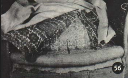
FIGURE 56. Turn the seam toward the front of the chair. Now pin the center of this seam to the center of the chair even with the back of the front edge roll.
