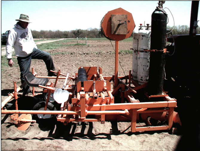
Fig. 2. A bed shaper that also inserts the drip tape, fumigates and lays the plastic in one pass.
