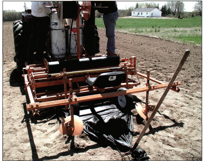
Fig. 9. Starting the mulch laying process by tying the plastic and tape to a pitchfork.
