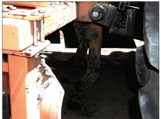
Fig. 10A and 10B. Fumigation equipment: fumigant tanks (A), fumigation knives (B).
