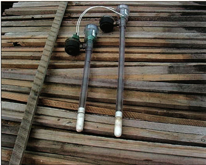
Fig. 12. A tensiometer used to measure soil moisture.
