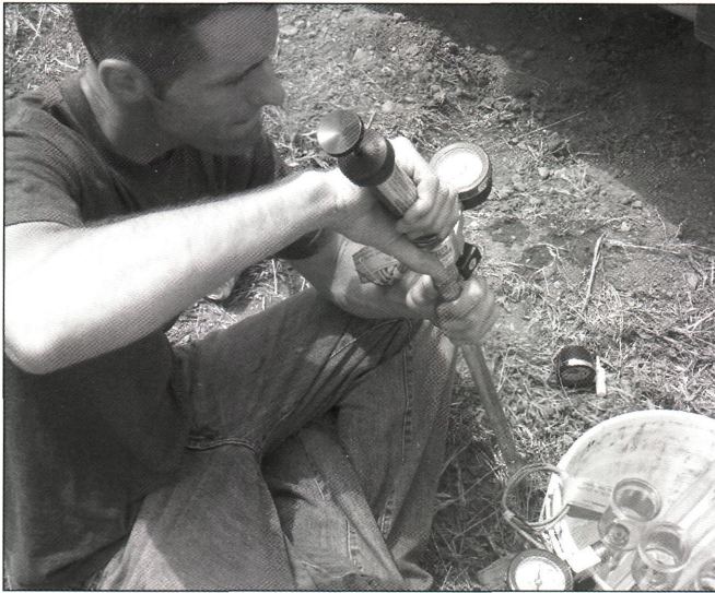
Fig. 5. MSU forestry graduate student Nick Gooch pumping a 24-inch tensiometer at one of our research locations in Michigan (photo by Pascal Nzokou, 2006).
