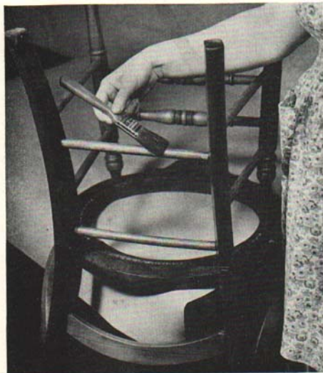
Fig. 7. Turn the piece of furniture upside down and apply the finish to the underneath parts first.
