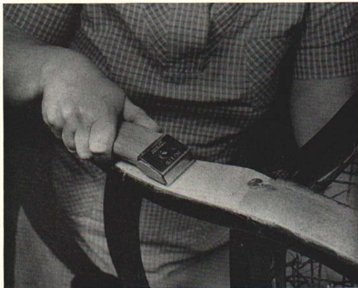
Fig. 3. A scraper is used to remove the old finish from flat surfaces.
