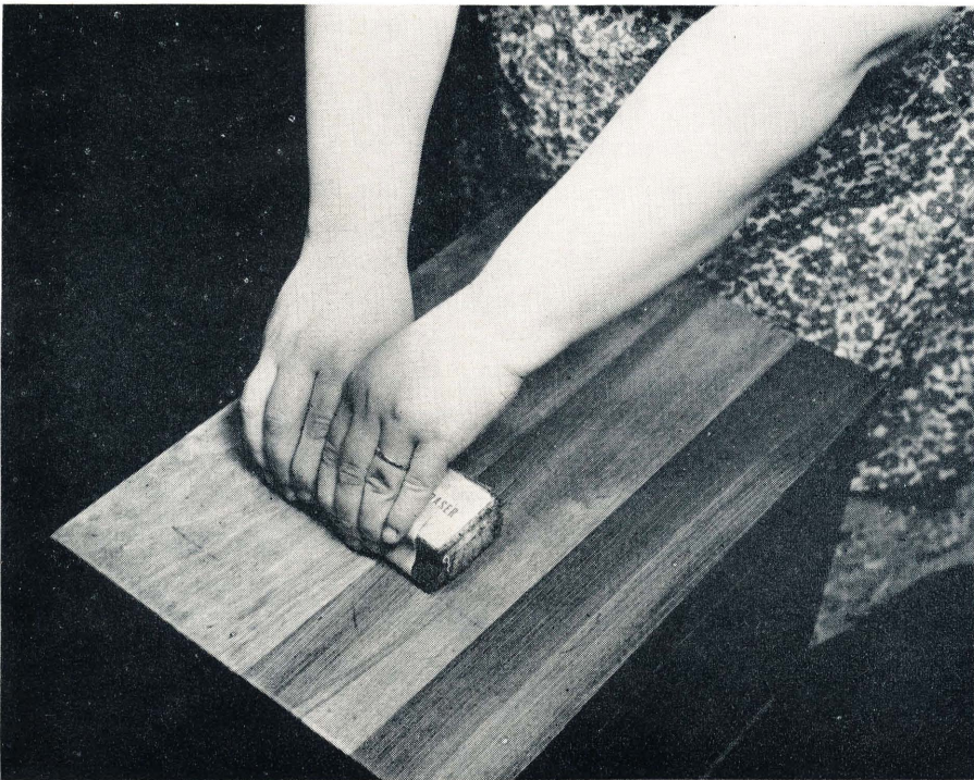
Fig. 6. A sanding block, for sanding large surfaces, can be made by wrapping the sandpaper around an eraser.
