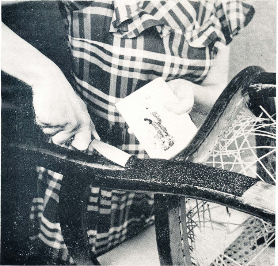
Fig. 1. Remove the old finish, which has been softened by a liquid remover, with a putty knife held firmly against the wood. Take care not to scratch the wood. The old finish can be wiped onto a newspaper which can then be burned immediately.
