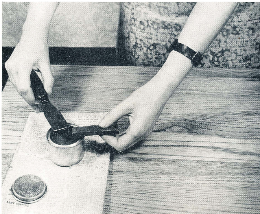
Fig. 4. Holes and large cracks are filled with stick shellac of matching color.
