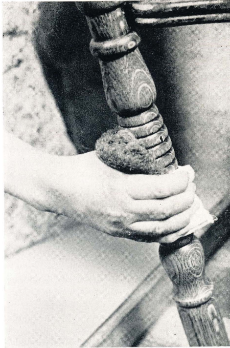
Fig. 2. Use steel wool and alcohol to remove the finish from turnings.
