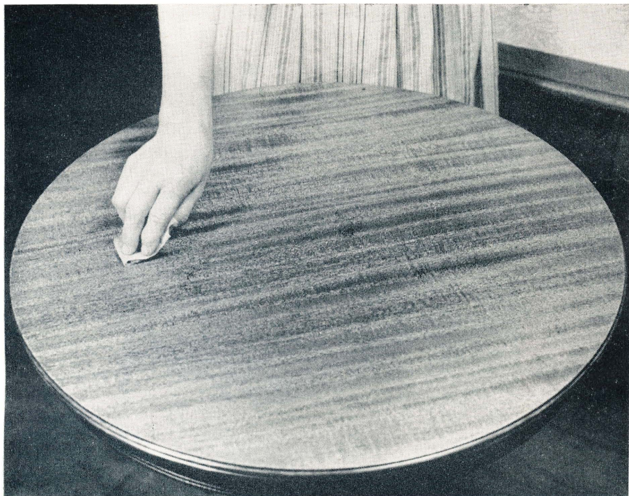
Fig. 8. Apply the penetrating seal liberally at first with a folded cloth. Rub the seal into the wood, going across the grain and finishing with the grain.
