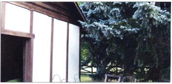
Figure 3. The spruce trees in this photo are located too close to the house. If they catch fire, they will likely create enough radiant heat to ignite the home. (Courtesy of MSU Extension.)
