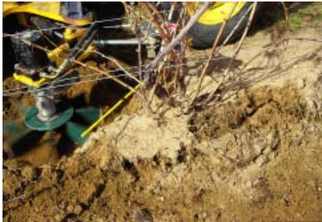
Fig. V-25, A. Paddle-wheel implement on a modified Weed Badger unit, custom-designed to remove soil around grapevines.
