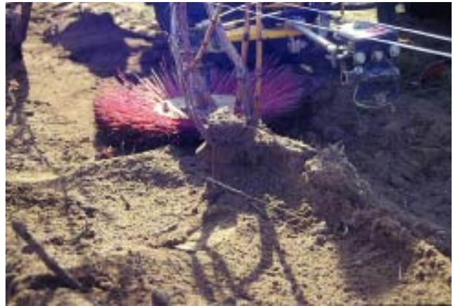
Fig. V-25, D. Side two removal of soil around Chardonnay vines with the custom brushing implement attached to a Weed Badger in spring 2004 at the MSU Southwest Michigan Research and Extension Center.
