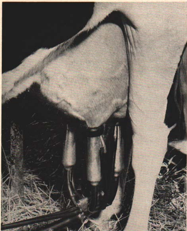
Fig. 5. This picture shows an undesirable practice of allowing the teat cups to crawl up on the udder as the cow milks out. When this condition occurs, the opening from the udder into the teat is closed. This allows the machine to irritate the internal lining of the teats—and may cause injury that will lead to infection. When milk is not flowing through the teat, the pull of the vacuum on the lining of the teat may also cause injury.
