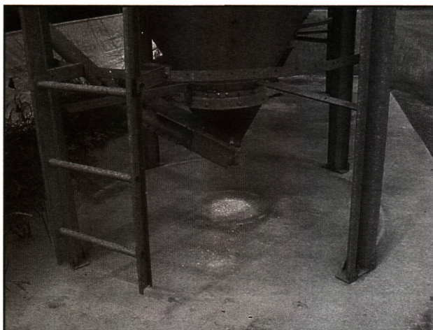
Figure 1. Reducing waste caused by equipment leaks can save feed and prevent rodents and insects.
