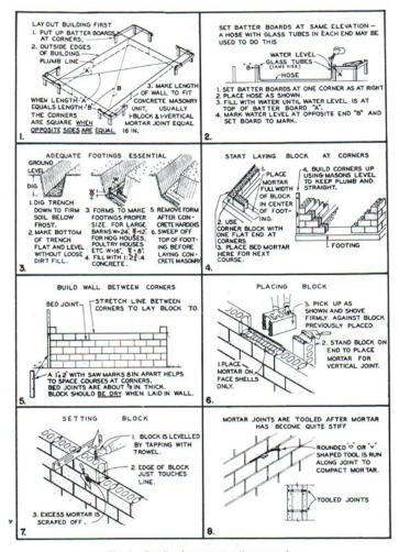
Fig. 5. Details of masonry wall construction.
