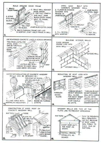
Fig. 5. Details of masonry wall construction-(Continued).
