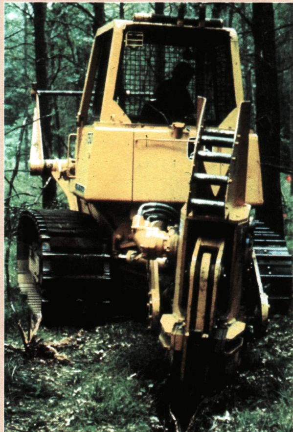
Figure 10 A vibratory plow with a 5-foot blade is most effective in severing root grafts between infected and healthy oak trees in locations where no underground pipes or cables are buried.
