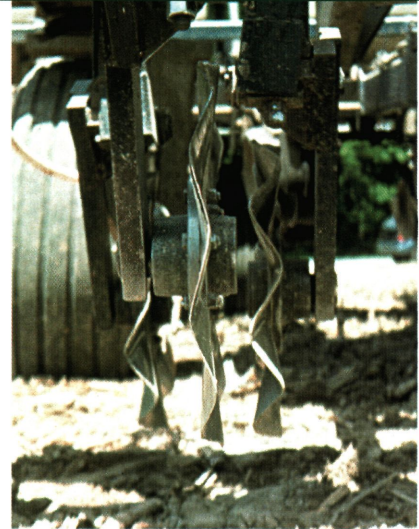
Close up of 3-coulters zone-till system.
