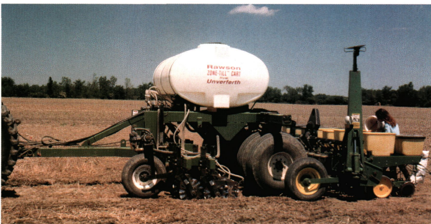
22-inch zone-till equipment with corn planter.
