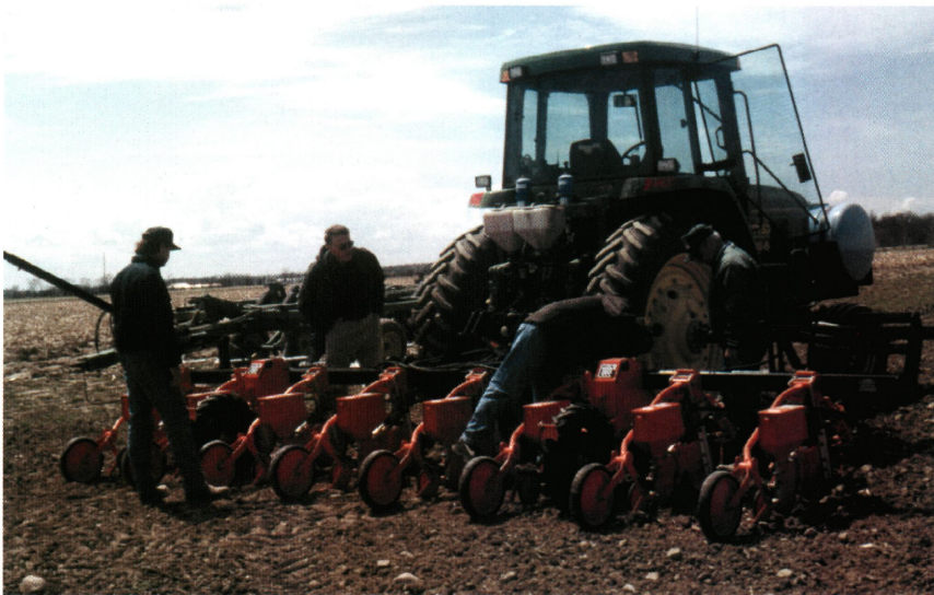
Zone-till equipment with specialized vegetable planter.
