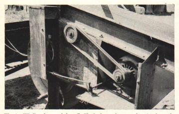
Fig. 4. Winding drum and shut-off. The brake can be seen where it rubs on the winding drum. Note the two gears which operate the automatic shut-off.
