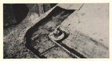
Fig. 15. Tightener idler. This idler is on an eccentric hub which is used in tightening the apron chain.
