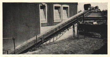
Fig. 16. The loading elevator on the Brook Brothers farm, Haslett, Michigan. This type is used on the double-gutter dairy barn in which an endless apron cleans the gutter and drops the manure onto the lower end of the loading elevator.
