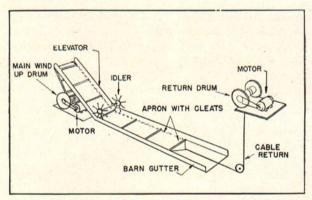
Fig. 1. Diagrammatic view of a "wind-up" type barn cleaner. Angle of elevator rise should not exceed 30°.
