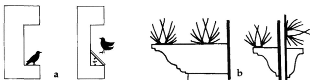
Figure 5. A board or metal covering over a ledge at a 45° angle (a) or porcupine wires (b) can be used to prevent roosting and nesting. (Figure by Renee Lanik, University of Nebraska-Lincoln.)
