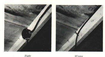
Fig. 4. Showing the proper way to support the lamp cord at the ceiling.
