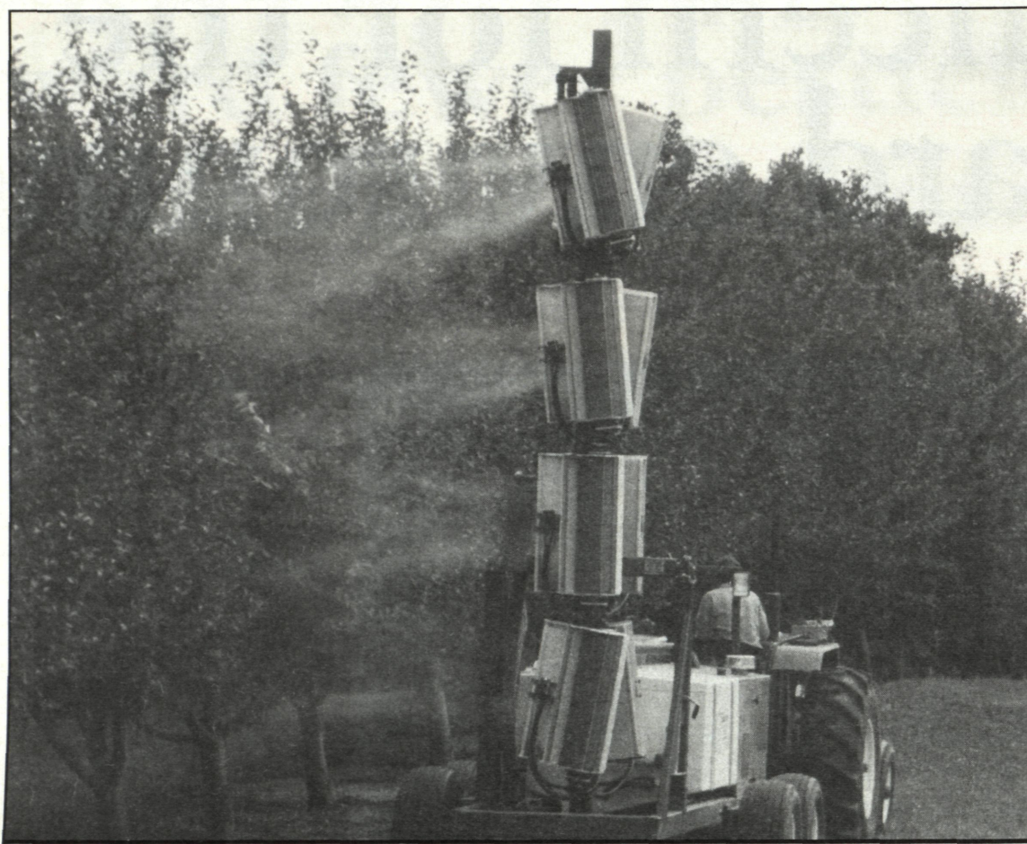
MSU's air curtain sprayer technology substantially reduces the amount of orchard chemical protectant that can escape into the atmosphere or fall to the ground by controlling the spray pattern into the tree. By contrast, the radial application pattern of conventional sprayers is prone to chemical drift.
