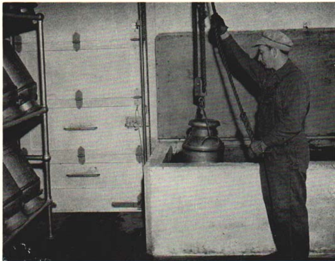
Fig. 7. The insulated concrete tank is most widely used in cooling milk. This dairyman has a device for conveying the cans of milk into and out of the tank. Note also his home-made can rack.
