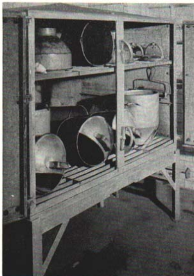
Fig. 6. Steam cabinet with doors ajar. Utensils here are effectively treated at 170° F. for 15 minutes. The heat then dries them promptly. They are protected here till the next morning.
