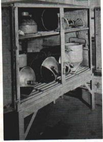
Fig. 6. Steam cabinet with doors ajar. Utensils here are effectively treated at 170° F. for 15 minutes. The heat then dries them promptly. They are protected here till the next milking.
