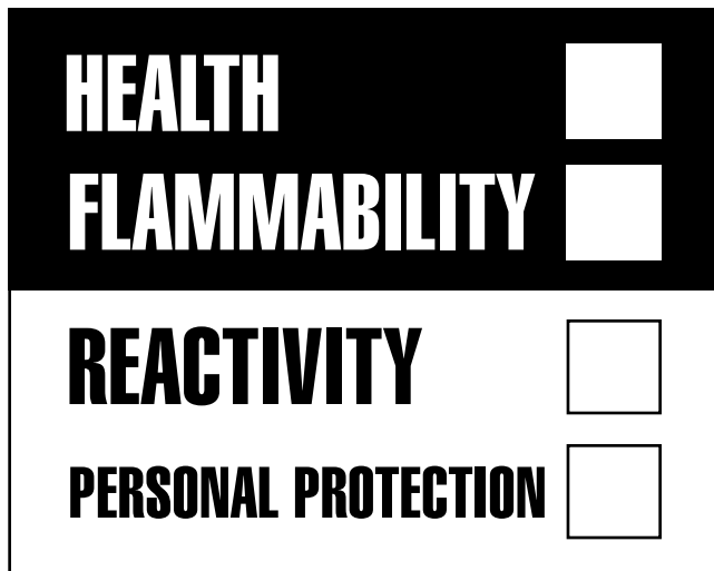
Example of a Hazardous Materials Identification System label.
