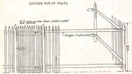
Fig. 25.—Poles must be close together and should be five feet or more high for a pole chicken run.
