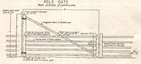
NOTE: Size of gate and poles used optional. Crosspieces can be neiled to end posts implace of fitted thru bore holes.
