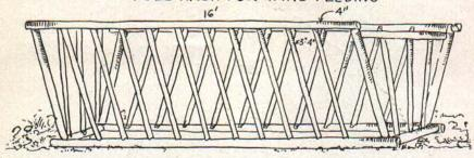
Fig. 42.—A pole rack for yard feeding. Can be made any size, but should be 15 or 16 feet long.
