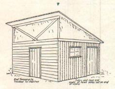
Fig. 17 (B)—First section of barn basement of hewn cedar posts, with temporary end and roof. End is covered with boards so that addition can be made easily.
