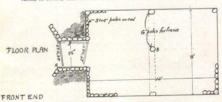
Fig. 20 (B)-Floor plan of root cellar.
