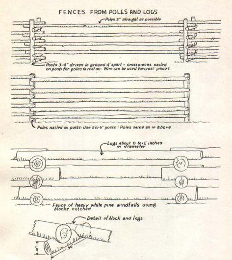
Figs. 26, 27 and 28.—Three types of pole fences commonly used. The fence in Fig. 28 (the bottom illustration) is made of old white pine deadfalls.
