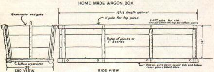
Fig. 35.—This wagon box is made of poles and boards or planks. It is easily made and will haul a big load.
