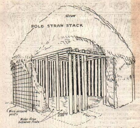
Fig. 44.—A pole frame, over which the straw is piled. The poles are close together on three sides, so that the cattle can eat from only one end. In this way, only one side has to be watched and kept covered.
