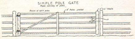
Fig. 32.—The simplest pole gate made. It is not as strong as those shown in Figs. 33 and 34,
