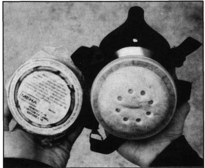
Pesticide-saturated filters and cartridges harm rather than protect applicators.
