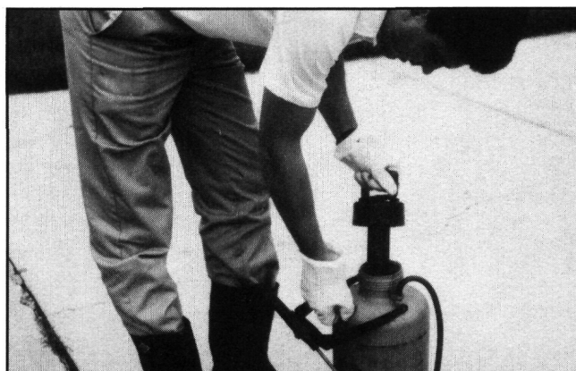
Small-capacity sprayers are used for spot treatments and small area applications.
