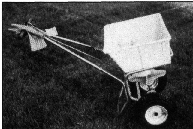
Granular spreaders are used to apply granular formulations of pesticide and fertilizer.
