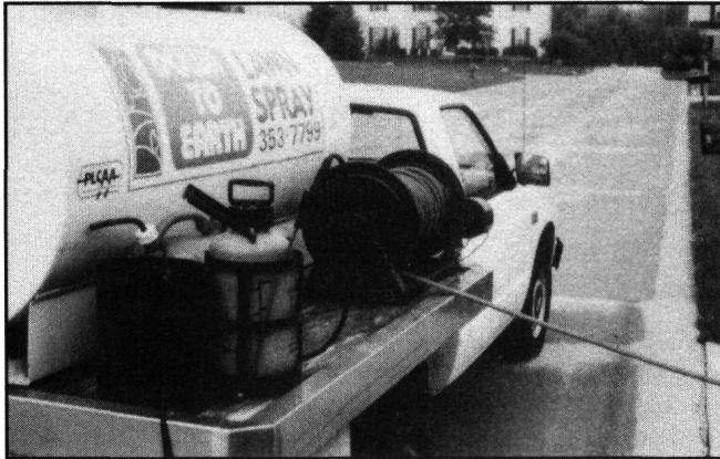
This pick-up truck, equipped with a hydraulic sprayer and large tank, is typical of the equipment used for large-volume lawn applications.
