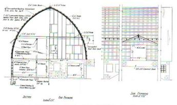
Fig. 34. Construction details of 36' x 60' Gothic type honey house.
