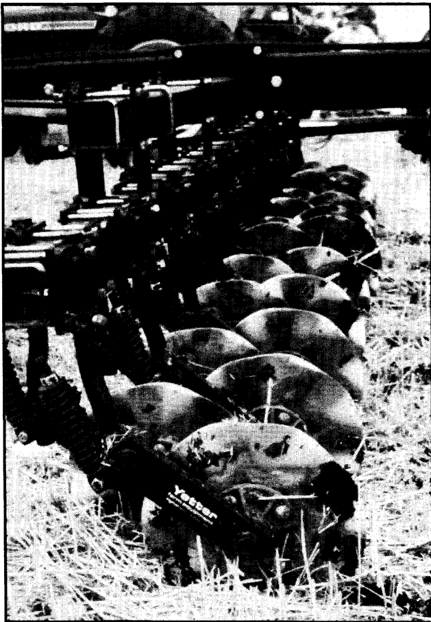
Fluted coulters till more soil than other types of coulters.
