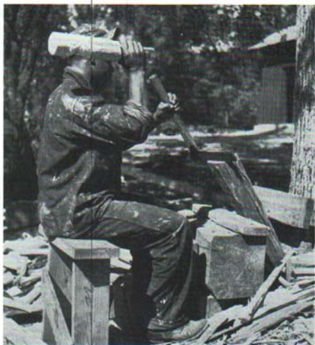
Fig. 16. Splitting out shakes with a shake-maker's froe. (Photograph by the U. S. Forest Service.)
