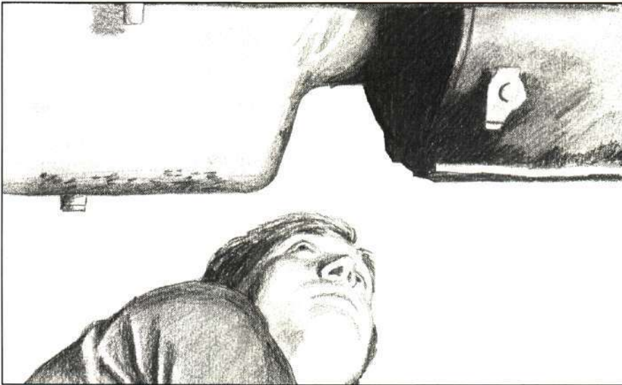
Check engine oil seals and ground under the oil pan for fresh oil
