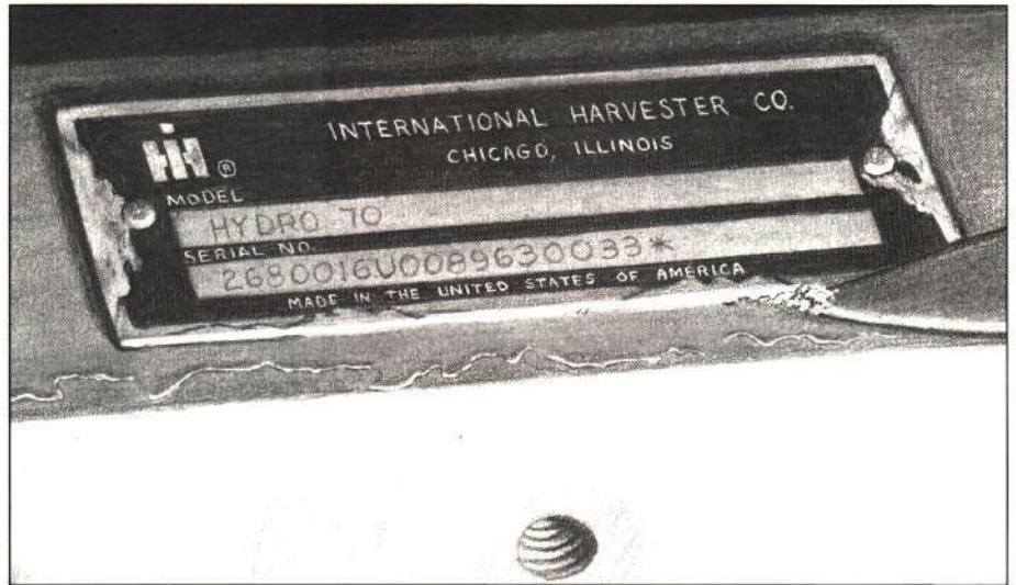
Make sure the PIN plate has not been tampered with
