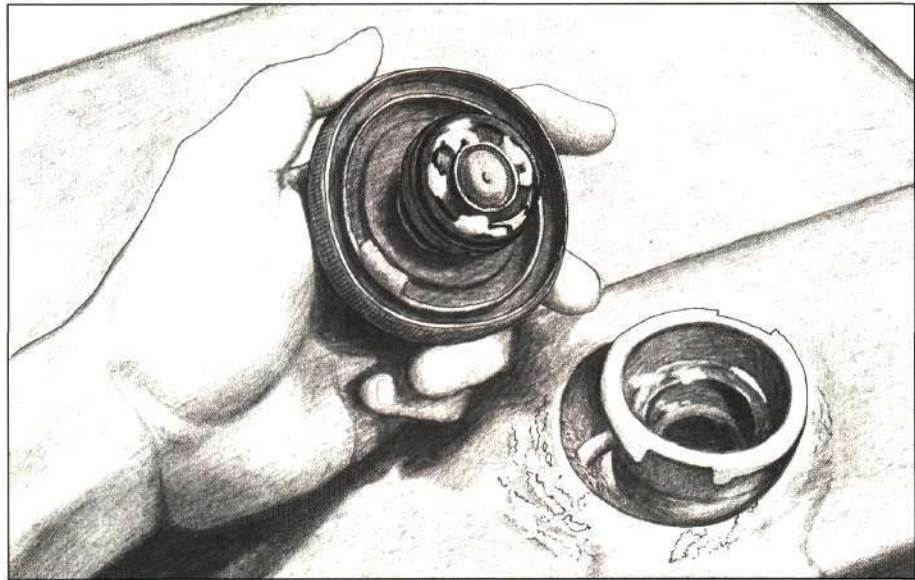
Creamy white deposits on the cap indicate oil in the coolant
