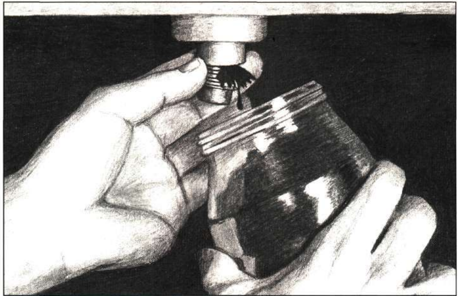
Collect and inspect oil samples when possible
