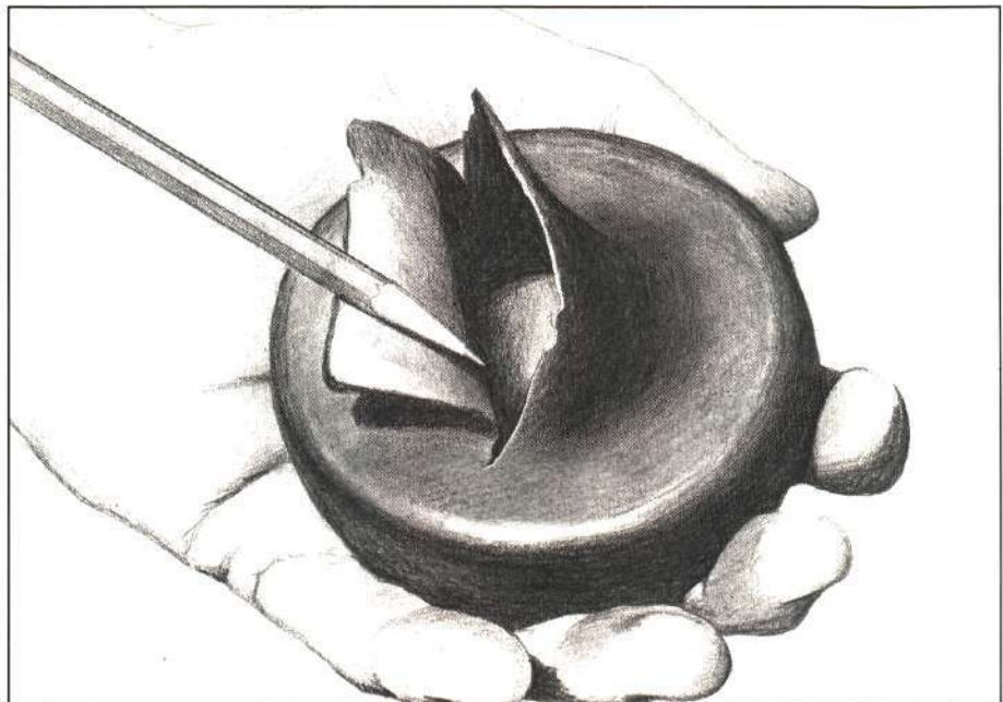
Torn dust unloader valve
