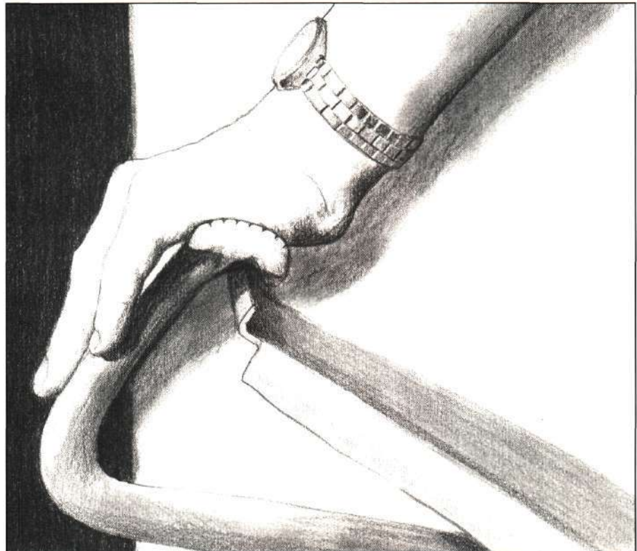
Check mechanical clutches manually
