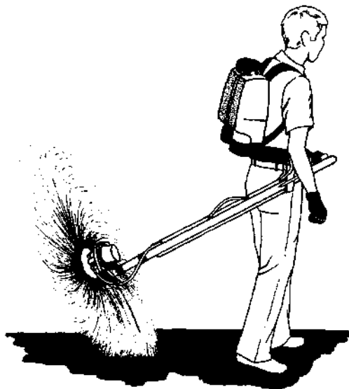
Controlled droplet applicator.
