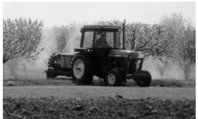
The trailer-mounted airblast sprayer uses a combination of air and liquid to deliver the pesticide to orchard trees.
