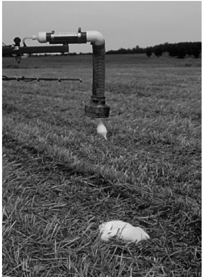
Foaming agents can be used for marking treated sections of a field.
