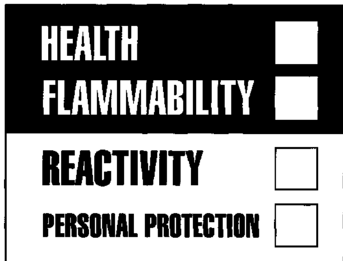
Example of a Hazardous Materials Identification System label.
